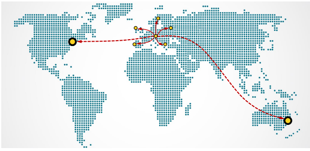
Figure 2: Dissemination overview: Blocks should be propagated to a few nearby and to a few distant nodes.
